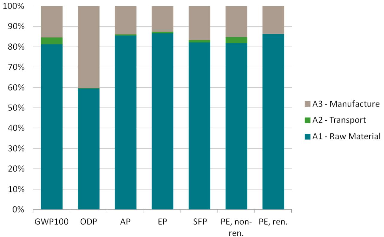
**Figure 4: Total life cycle impacts of 93 square meters (1,000 sq ft) of MCM panel, TRACI 2.0 impacts and primary energy inventory**
