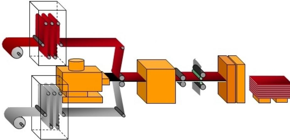
Figure 1: Schematic of MCM Laminating Process
