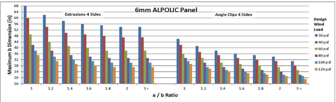
\* Controlled by maximum allowable bending stress (13,200psi) or maximum panel deflection ( $b/60$ ) as applicable.
