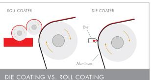
Although widely used roll coaters can achieve adequate quality and efficiency, our advanced die coaters permit direct coating on the aluminum surface to ensure smoother, finer finishes without roping marks.
